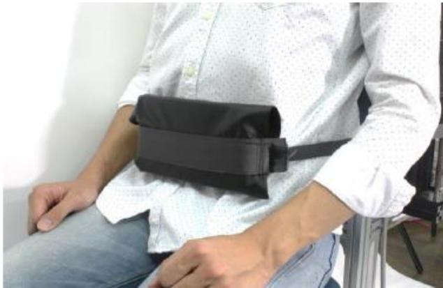
Figure 3. The abdomen pressing part of the belt-driven assistive robot.
